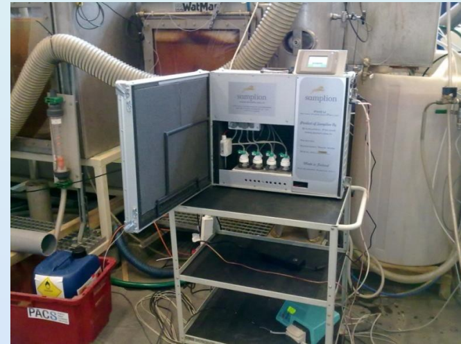
Coliline PMEU with Automated Sample Collection System
